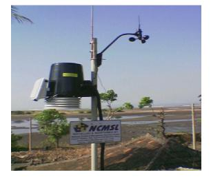
Figure-3: Automatic Weather Stations (AWS)
