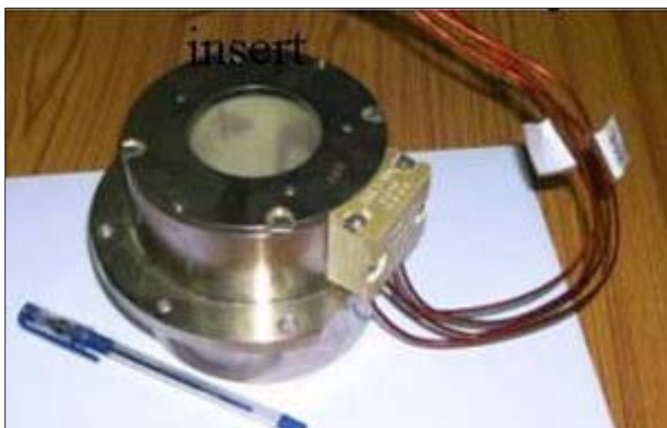
One of the 616 superconducting MCDO magnets supplied to CERN by RRCAT
