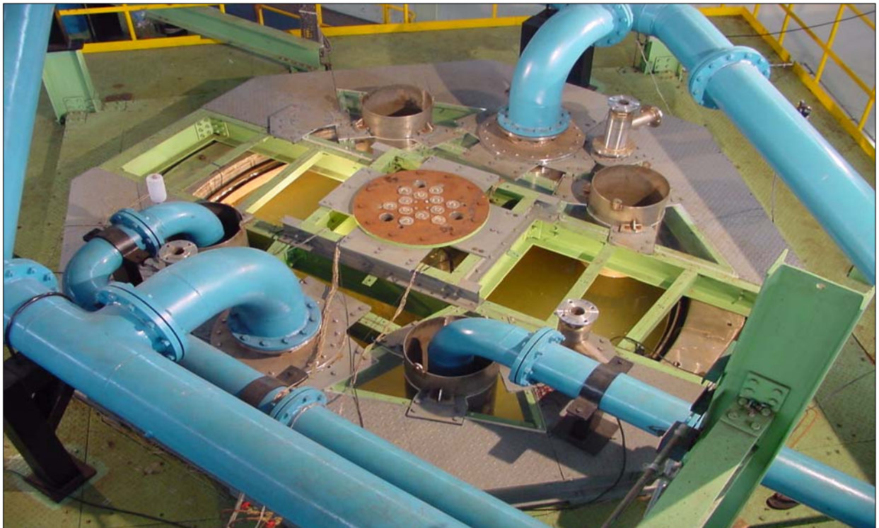
Top view of 1/4 th Reactor Assembly Model. The set up has been erected. Various Thermal Hydraulics Experiments will be carried out using the above facility.
