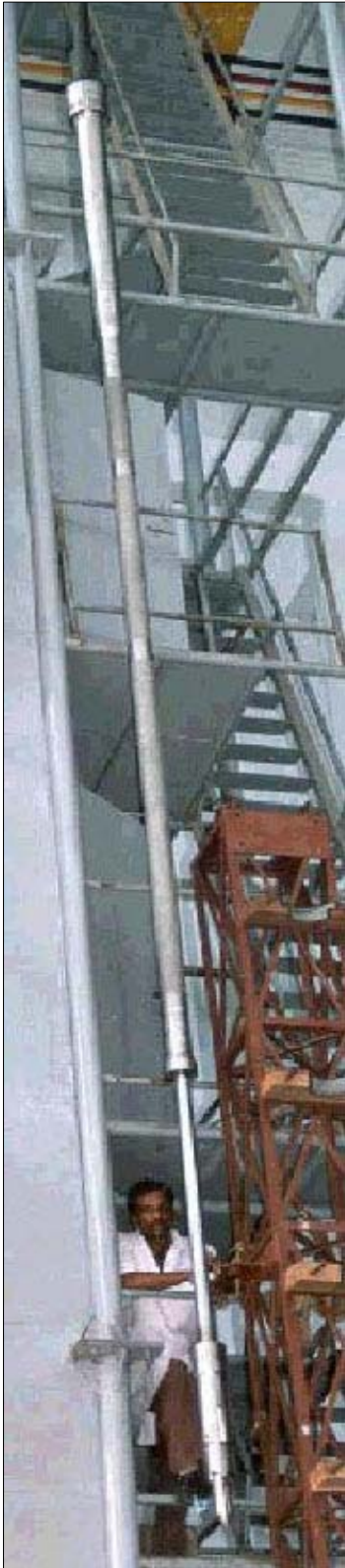
Testing of Control and Safety Rod Drive Mechanism (CSRDM) in Sodium for Prototype Fast Breeder Reactor
