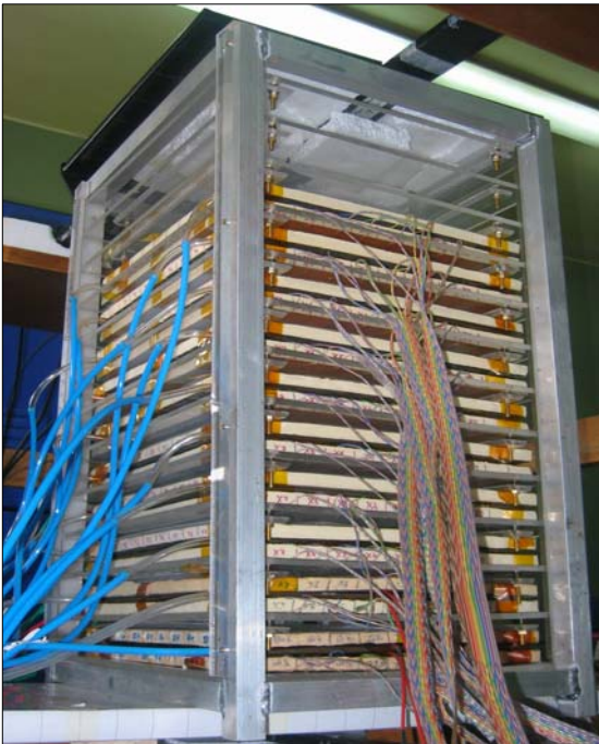
Stack of 10 Resistive Plate Chambers (RPC) as active detector element for Muon tracking
