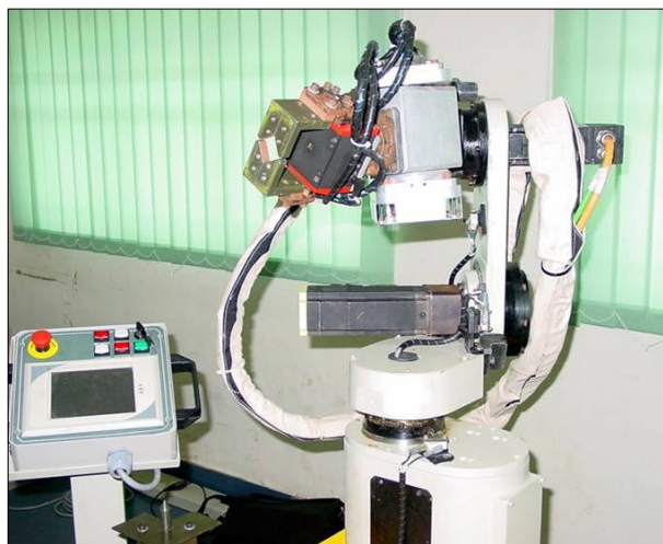
Desk-top Articulated Robot with 6 degrees-of-freedom developed at IGCAR for studying fuel pellet handling, remote repairs and decontamination
