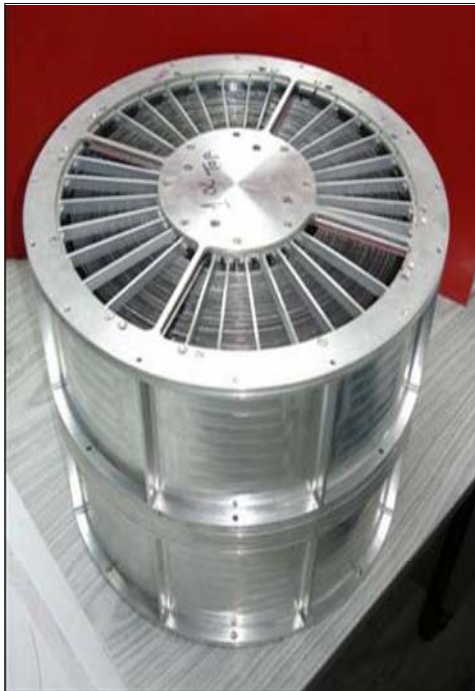
Of the three payloads for Astrosat mission of ISRO two are being piloted by teams from TIFR. Picture shows the soft X-ray telescope mirror assembly for the X-ray payload.
