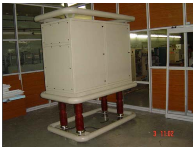
High voltage platform for the Accelerator Driven Sub-critical System (ADS) ion source at VECC
