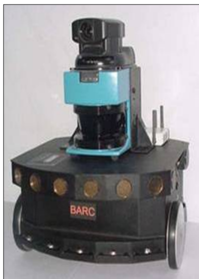
Mobile robot for remote survey and inspection developed at BARC
