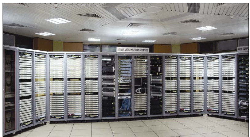
BARC's supercomputing facility : Tera Flop Class 512 Node Anupam-Ameya Supercomputer
