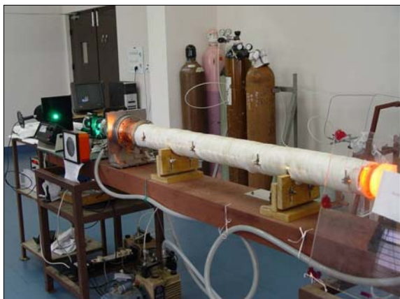
25 Watts CuBr Laser developed at RRCAT
