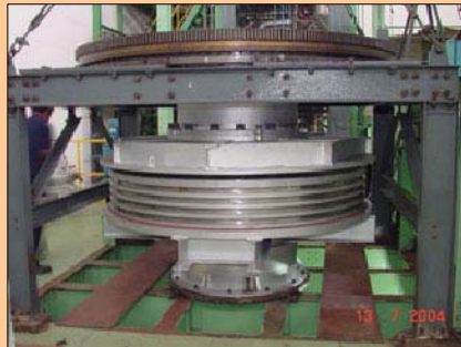
Inflatable seal testing facility for FBTR and PFBR seals
