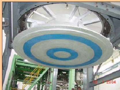
Inflatable seal testing facility for FBTR and PFBR seals
