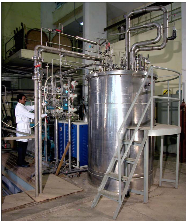
Indigenously developed Cryogenic (Helium) Refrigeration System at BARC
